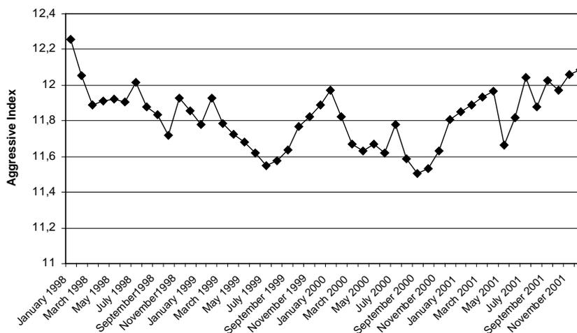
Fig. 1. Aggressive Indices calculated for finished water produced by the Dobczyce Reservoir WTP – based on data provided by the local waterworks company
