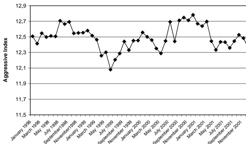
Fig. 2. Aggressive Indices calculated for finished water produced by the Rudawa River WTP – based on data provided by the local waterworks company
