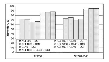
Fig. 6. Determination of the retention coefficient of TDS and TOC for the solutions investigated. Feeds: KCl – solutions in two concentrations of KCl, TDS and TOC – retention coefficient of TDS or TOC, GL40 – solution of glucose in a constant concentration (40 mg C/dm<sup>3</sup>), KCl + GL40 – solutions of KCl with glucose
