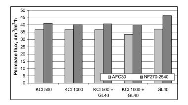
Fig. 5. Determination of permeate flux when the solution of KCl with or without glucose was the feed. The feeds: KCl – solution of KCl in two concentrations, GL40 – solution of glucose in a constant concentration equal to 40 mg C/dm<sup>3</sup>, and KCl + GL40 – the solution of KCl with glucose
