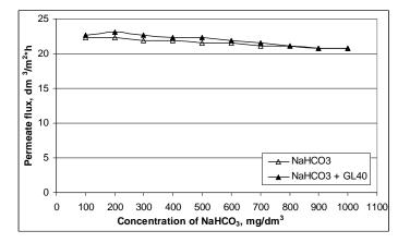
Fig. 3. The dependence of the permeate flux on the concentration of inorganic salt. The feeds: aqueous solution of NaHCO<sub>3</sub> and aqueous solution of NaHCO<sub>3</sub> with glucose addition
