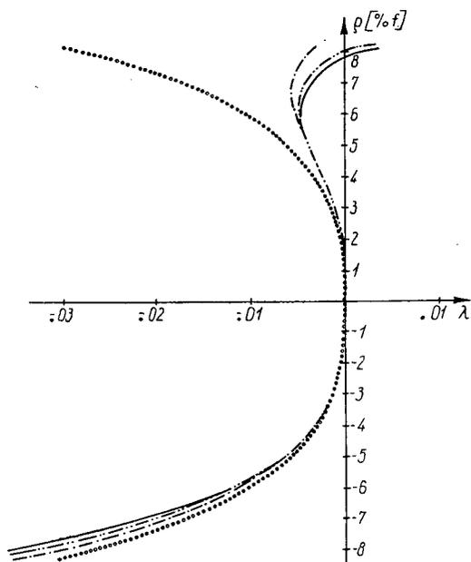
Fig. 1c. The graphs of the wave aberration for the field angle  $12^\circ$
