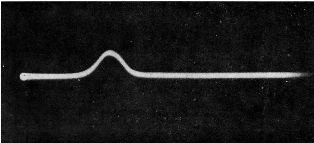
Fig. 1. Picture of a giant laser pulse of 40 ns total duration
