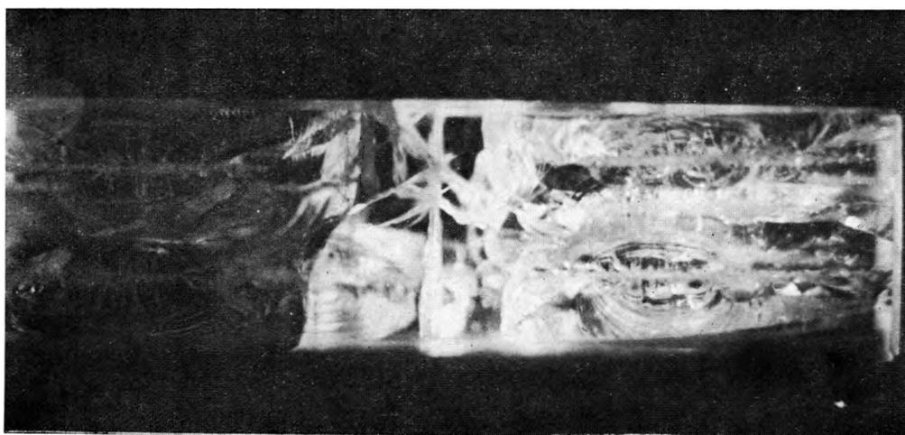
Fig. 3. KDP crystal, completely damaged by several laser shots, each of a flux density of the order of 100 GW/cm<sup>2</sup>
