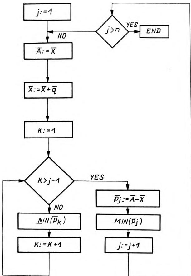
Fig. 2. Flow diagram of minimization procedure
