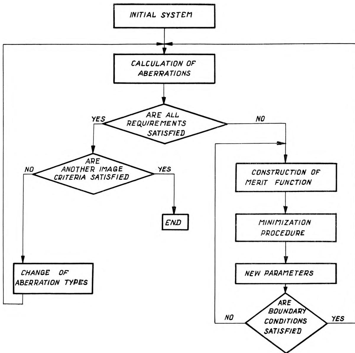
Fig. 1. A general flow diagram of the optimization method
