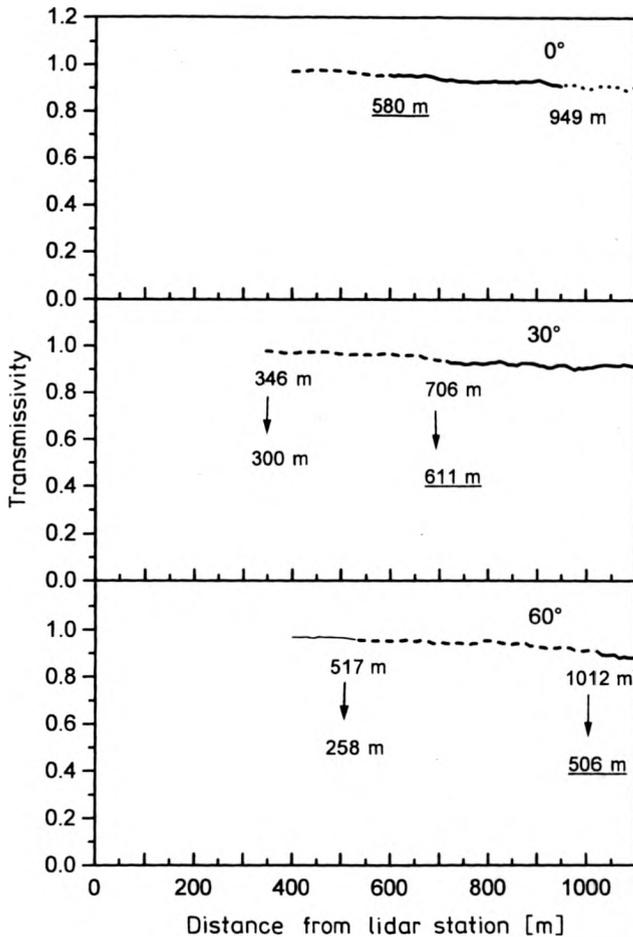
Fig. 4. Transmissivity profiles at three different zenithal angles. The same range in the vertical direction has been indicated by the same line type. The arrows indicate the corresponding height along the vertical direction.
