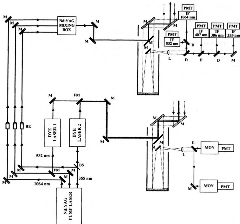
Fig. 1. Experimental setup. BE — beam expander, D — dichroic mirror, FM — flipper mirror, IF — interferential filter, MON — monochromator, M — mirror, BS — beam splitter, L — lens.
