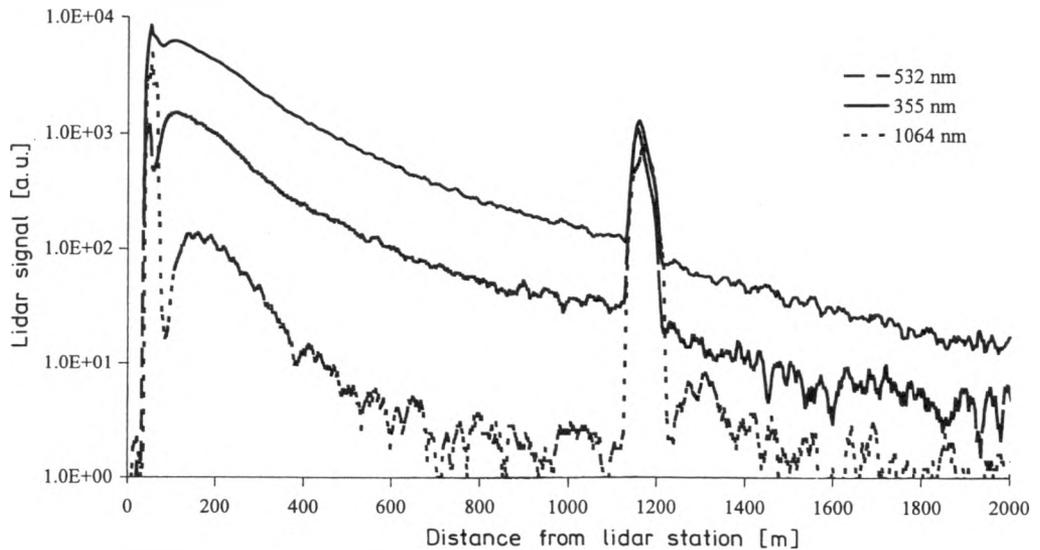
Fig. 7. Lidar echoes from the stack emission plume at three different laser wavelengths.
