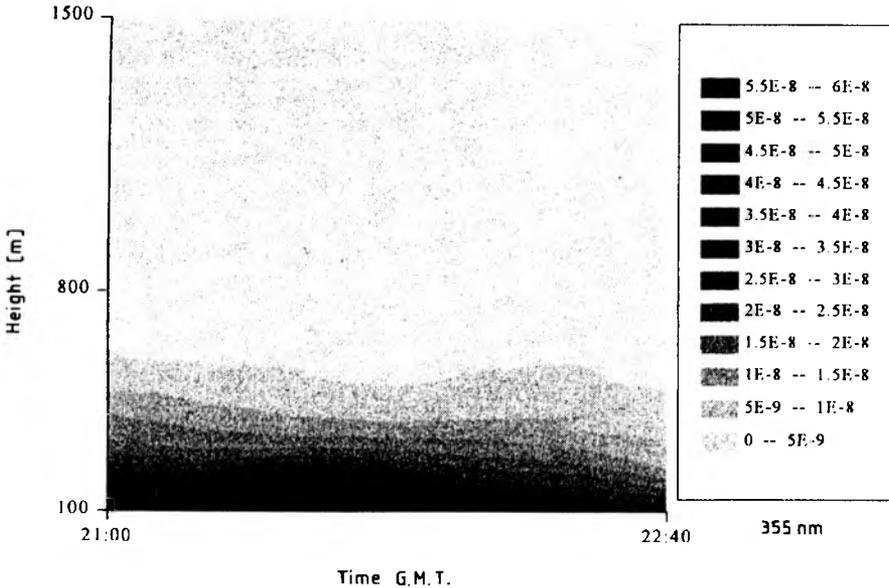
Fig. 2. Temporal evolution of the backscattering coefficient at 355 nm (Tito Scalco, February 11, 1998).
