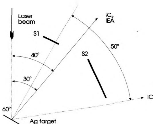
Fig. 6. Experimental arrangement for testing the implantation of ions from the laser plasma in different materials.
