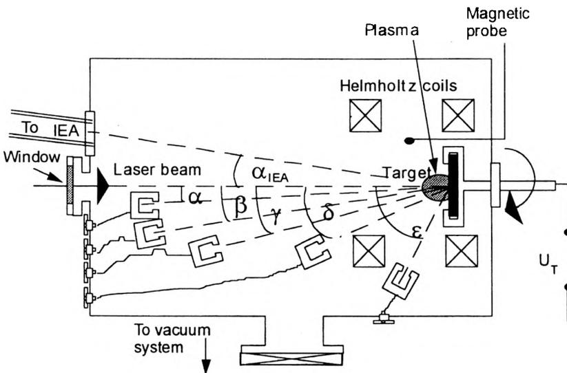
Fig. 4. Experimental setup (not in scale) for studies of the effect of magnetic field on the ion beam emitted from the laser plasma.
