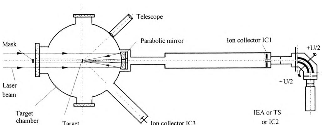
Fig. 1. Experimental setup at the IP ASCR in Prague with the mirror focusing system for studies of ion streams from the high Z-plasma.
