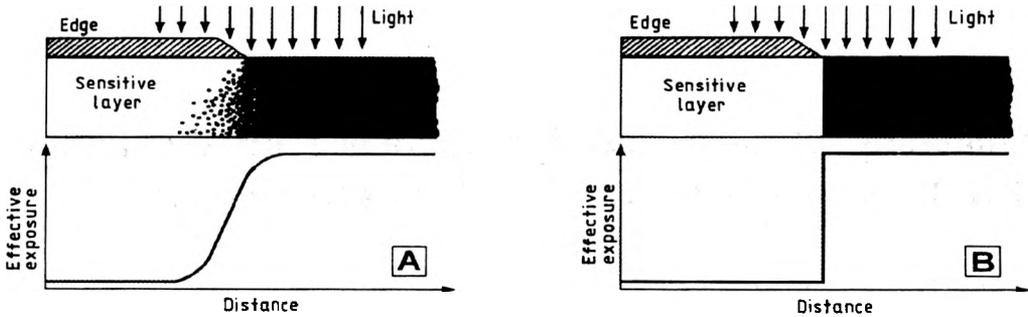
Fig. 1. Distribution of the effective exposure in the light sensitive layer at the image-background border (fields of strong and weak irradiation) shown for two cases: **a** – when light scattering effect occurs within the heterogeneous light sensitive layer, **b** – for the lack of light scattering effects.
