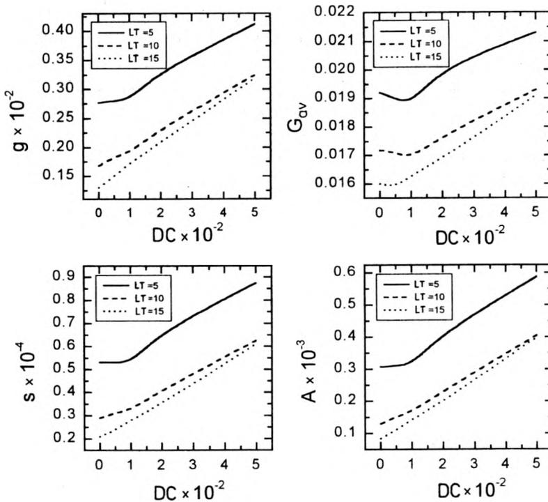
Fig. 6. Changes in the contour sharpness indicators as a function of acutance dye concentration in the light sensitive layer of thickness 5, 10, 15  $\mu\text{m}$ .  $G_{uv}$  denotes the average gradient of the border curve,  $g$  denotes the sharpness indicator suggested by Jones and Higgins, while  $s$  — that proposed by Müller and  $A$  — that proposed by Perrin.
