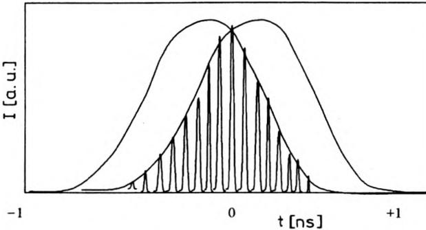
Fig. 1. Modulations of two overlapped chirped pulses.
