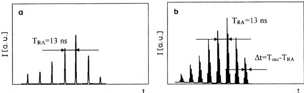
Fig. 6. Train of pulses in the output of the RA upon injection of a single pulse into the RA (a). Train of pulses in the output of the RA upon injection of a pulse train into the RA (b).
