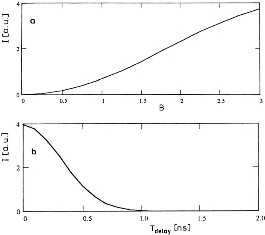
Fig. 3. Increase of first satellite intensity with  $B$ -integral under conditions of Fig. 2 (a). Decrease of first satellite intensity with time delay between main pulse and postpulse under conditions of Fig. 2 (b).
