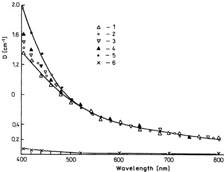
Fig. 1. Spectral dependence of optical density for the porous glass DV-1M after irradiation with  $\gamma$ -quanta of  $^{60}\text{Co}$  at different exposure doses: 1 – original glass, 2 –  $10^5$  R, 3 –  $10^6$  R, 4 –  $10^7$  R, 5 –  $10^8$  R, 6 – the same for the porous glass impregnated with silicon-organic polymer at the  $\gamma$ -quanta of  $^{60}\text{Co}$  exposure dose of  $10^8$  R.
