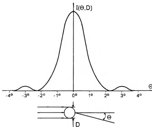
Fig. 2. Intensity distribution  $I(\theta, D)$  of the light scattered by a drop of diameter  $D = 20 \mu\text{m}$  illuminated by a plane wave of wavelength  $\lambda = 0.63 \mu\text{m}$  depending on the observation angle  $\theta$ .
