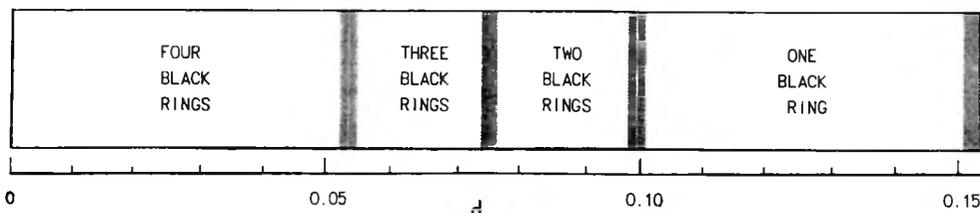
Fig. 11. Number of dark rings  $p$  visible in the diffraction image as dependent on relative standard deviation  $d$ .
