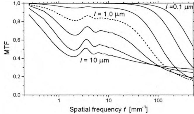
**Fig. 8.** The MTF of the light-sensitive system with AH layer for variable average free paths of the photon,  $l = 0.1, 0.2, 0.5, 1, 2, 5$  and  $10 \mu\text{m}$ .
