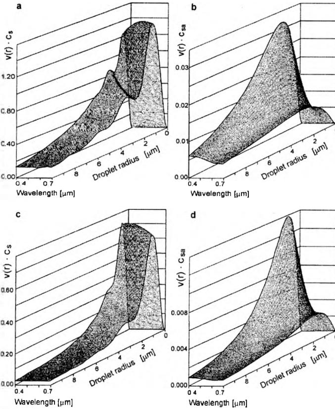
Fig. 4. Distributions of attenuation cross-sections (a) and (c) and absorption cross-sections (b) and (d) versus radius of suspension of crude oil type Romashkino after one weak of aging (a) and (b), after two weeks of aging (c) and (d).
