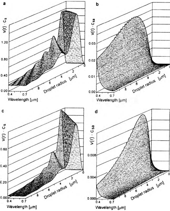
Fig. 5. Distributions of attenuation cross-sections (a) and (c), and absorption cross-sections (b) and (c) versus radius of suspension of crude oil type Petrobaltic after one week of aging (a) and (b), after two weeks of aging (c) and (d).
