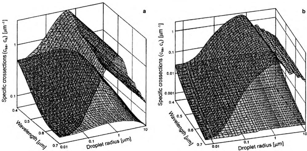
Fig. 3. Specific light attenuation cross-sections  $c_{\text{att}}$  (left surfaces) and absorption  $c_{\text{ab}}$  (right surfaces) for suspension of crude oil types Romashkino (a) and Petrobaltic (b).
