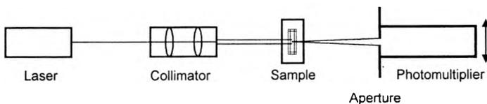
Fig. 1. Scheme of experimental setup.
