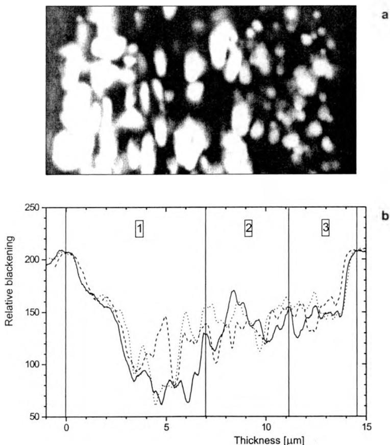
Fig. 2. Microscopic image of the cross-section of the light-sensitive layer of the Konica Monochrome VX 400 negative. Magnification  $5000\times$  (a). Averaged image blackening profile for light-sensitive layer cross-section of Konica Monochrome VX400. 1, 2, 3 — fluctuation areas corresponding to the layers of the light-sensitive emulsion differing from each other by the magnitude of the spherical crystals of AgHal (b).
