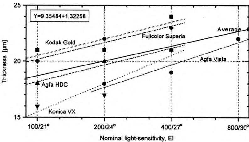
Fig. 4. Relation between the total thickness of the light sensitive emulsion layer and the nominal exposure index determined for a group of light-sensitive materials under examination.
