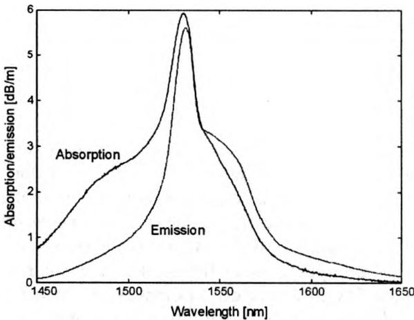
Fig. 2. Absorption and emission of a typical fibre given in Tab. 1.
