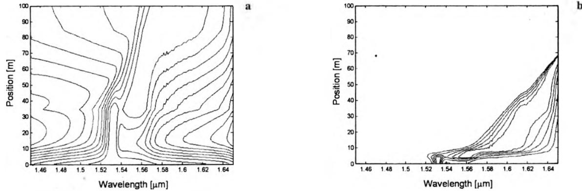
Fig. 5. Propagation of ASE noise in the forward (a) and backward (b) direction. The ASE noise power at a given position in the fibre was normalised to the maximum power of an ASE wavelength at this point. The z-axis is logarithmic. The EDF is 100 m long, the signal wavelength and pump wavelength is 1.60 μm and 0.98 μm, respectively. The signal power is 1 mW and the pump power is 100 mW.
