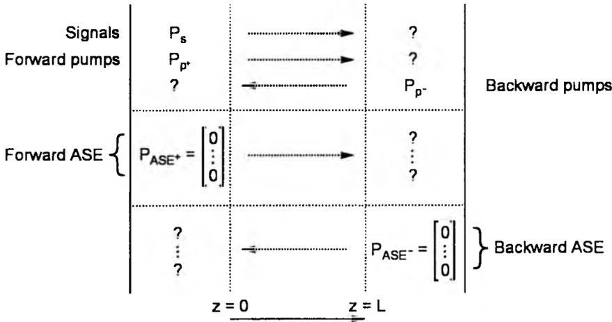
Fig. 1. Boundary conditions in EDFA. Dashed line arrows indicate propagation directions of light beams.
