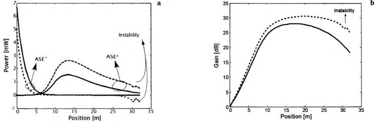
Fig. 4. Influence of the stabilization procedure on solution. The bold lines indicate solution after stabilization. Forward and backward ASE as a function of position in the fibre (a) and the gain as a function in the fibre (b).
