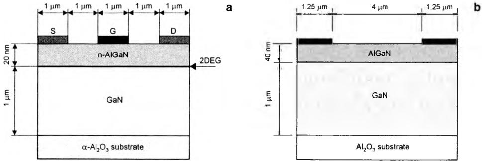
Fig. 1. Schematic cross-section of modelled devices: HFET (a), MSM (b).
