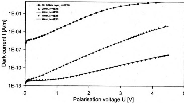
Fig. 6. Influence of AlGaIn layer thickness and background electron concentration  $N$  [ $\text{cm}^{-3}$ ] on photodetector dark current.
