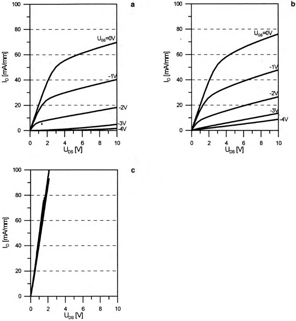
Fig. 4. HFET output characteristics depending on electron concentration in GaN buffer:  $1 \times 10^{14} \text{ cm}^{-3}$  (a),  $2 \times 10^{15} \text{ cm}^{-3}$  (b),  $1 \times 10^{17} \text{ cm}^{-3}$  (c).
