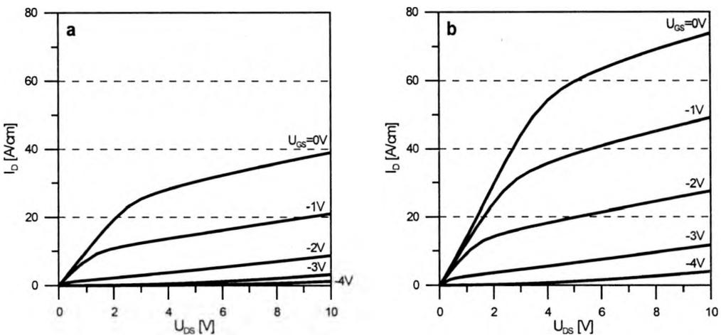
Fig. 5. HFET output characteristic without (a) and with (b) piezoelectric effect.
