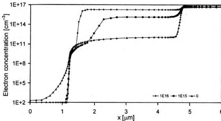
Fig. 7. Electron concentration under the AlGaIn layer ( $1 \text{ kW/m}^2$  incident light), depending on background electron concentration in GaN buffer ( $U = 3 \text{ V}$ ).
