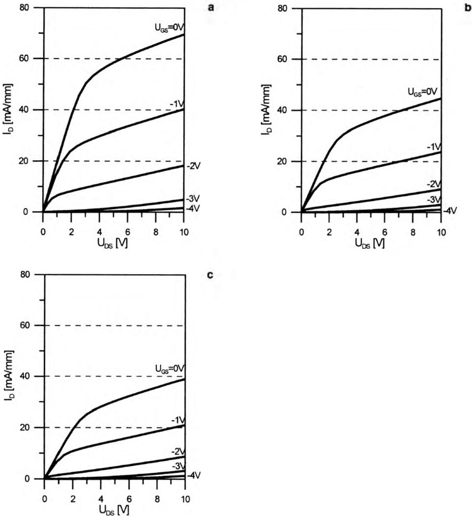
Fig. 3. HFET output characteristics depending on AlGaIn layer thickness: 20 nm (a), 35 nm (b), 50 nm (c).
