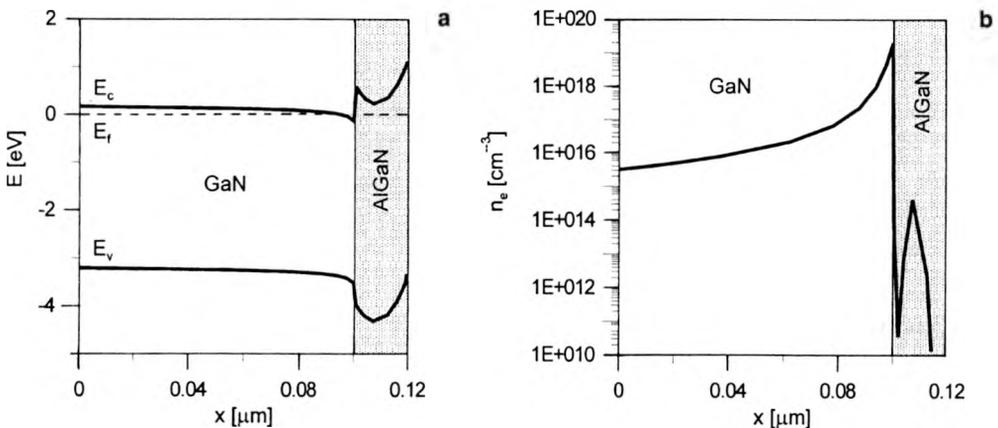
Fig. 2. Band diagram (a) and electron concentration (b) at the heterostructure (HFET, equilibrium).
