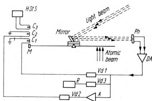
Fig. 1. Block scheme of the microbalance electronic part
