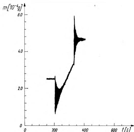
Fig. 2. The record of the mass  $m$  of indium atoms deposited on the microbalance scale; the jump  $s$  caused by atomic momentum in the beam is visible
