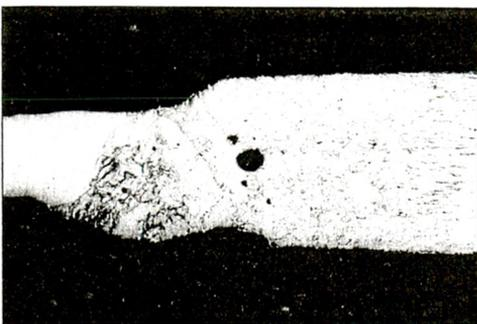
▲ Fig. 6. Macrostructure of weld of W-Mo. Magnification  $30\times$ .
