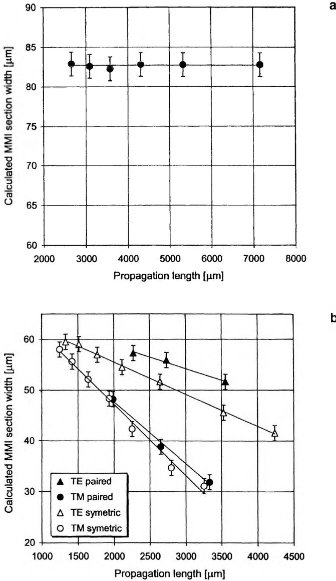
Fig. 11. Dependence of calculated MMI section width on the propagation length; **a** – MMI section of the width 81  $\mu\text{m}$ , made by  $\text{Ag}^+\text{-Na}^+$  ion exchange, **b** – MMI section of the width 60  $\mu\text{m}$ , made by  $\text{K}^+\text{-Na}^+$  ion exchange.
