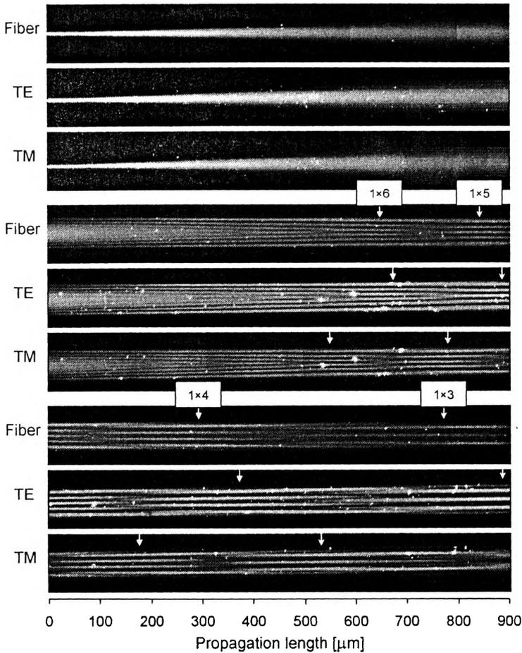
Fig. 6. Successive sequences of recorded mode field interference images for MMI section of the width  $60\ \mu\text{m}$ , made by  $\text{K}^+\text{-Na}^+$  ion exchange, symmetrically excited.
