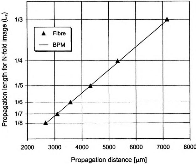
Fig. 8. Comparison between experimental and theoretical dependences of propagation lengths for  $N$ -fold images on the propagation distance; MMI section of the width  $81 \mu\text{m}$ , made by  $\text{Ag}^+\text{-Na}^+$  ion exchange, excited at one third of the section width.
