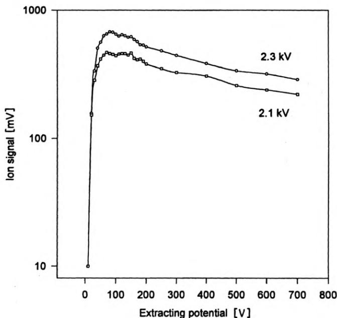
Fig. 3. Ion yield versus extracting potential
