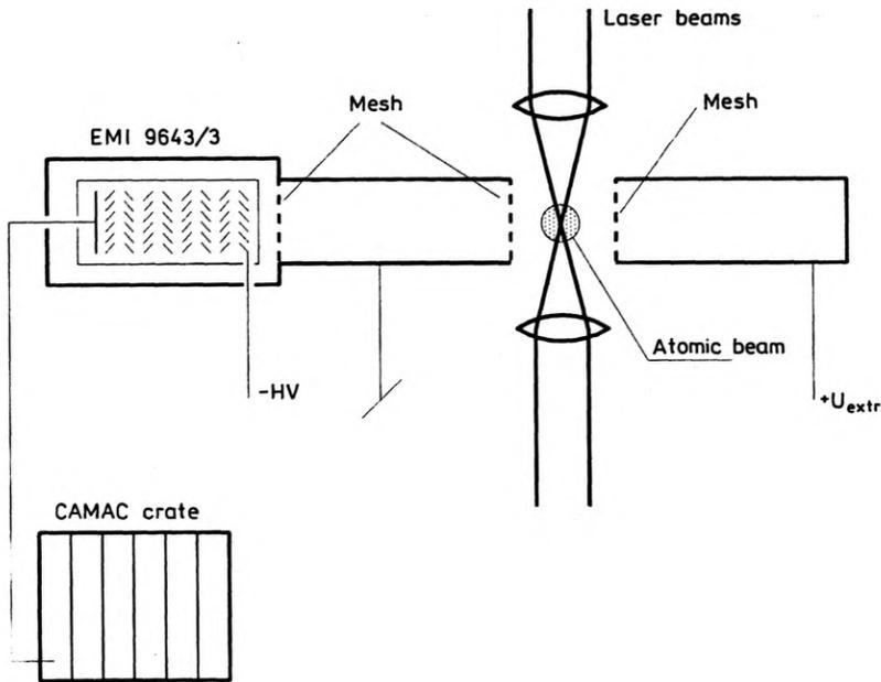
Fig. 2. Ion detection unit
