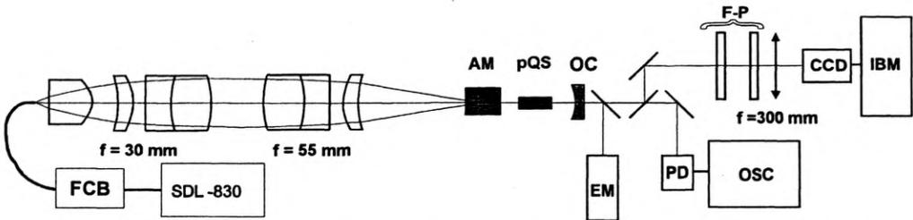
Fig. 1. Scheme of experimental set up SDL-830 – laser diode driver, FCB – fiber coupled diode bar, AM – active medium Nd:YAG crystal, pQS – LiF:[F<sub>2</sub><sup>-</sup>] crystal with initial transmission 65%, OC – output coupler with 10% transmission and 200 mm radius of curvature, EM – energy meter, PD – photodetector, F-P – Fabry–Perot interferometer with basis of 10 mm, CCD – CCD camera, IBM – PC computer 486, OSC – digital or analog oscilloscope
