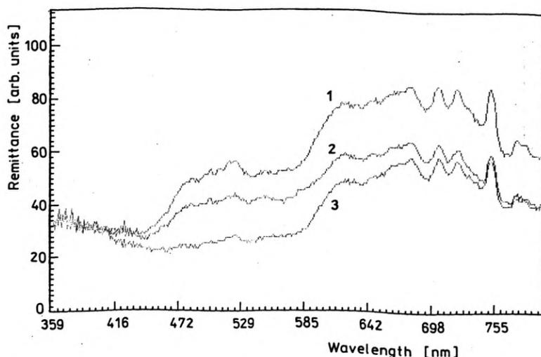
Fig. 5. Remittance spectra of: 1 — light-blue blood vessel under the skin, 2 — gel sallow, and 3 — reddish skin burn
