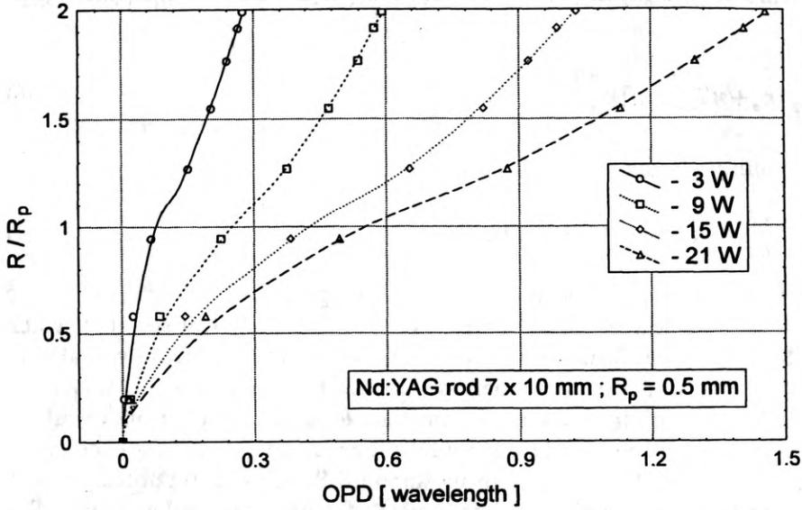
Fig. 2. OPD versus radius of incident rays for several values of pump power; Nd:YAG rod  $7 \times 10$  mm, pump radius 0.5 mm, with parabolic component
