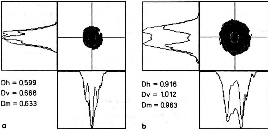
Fig. 7. Beam intensity distribution for the Nd:YAG laser: a — Bessel-like shape at a distance of 480 mm from the lens, b — annular-like shape at a distance of 520 mm from the lens
