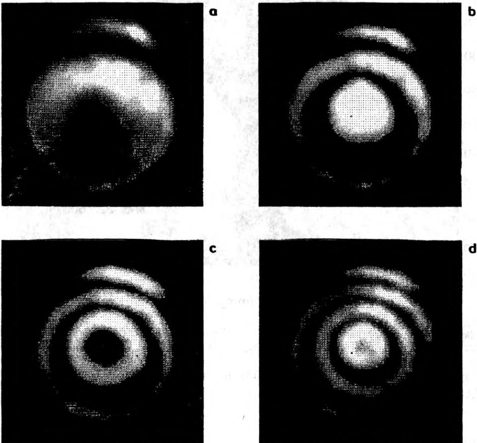
Fig. 4. Interferograms of thermally induced wavefront aberration of Nd:YAG rod  $7 \times 10$  mm for several values of pump power: a — 2.7 W, b — 5.2 W, c — 7.5 W, d — 10.2 W
