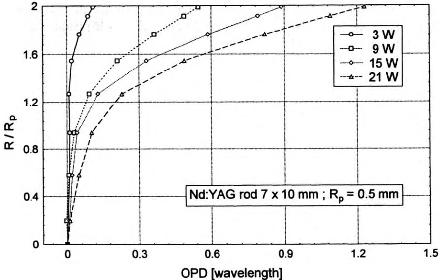
Fig. 3. OPD versus radius of incident rays for several values of pump power; Nd:YAG rod  $7 \times 10$  mm, pump radius 0.5 mm; after removing parabolic component
