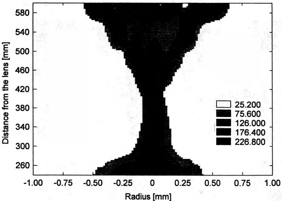
Fig. 6. Beam intensity distribution as a function of the distance from the lens of focal length 300 mm; Nd:YAG laser with  $7 \times 10$  mm rod at 8.8 W pump power
