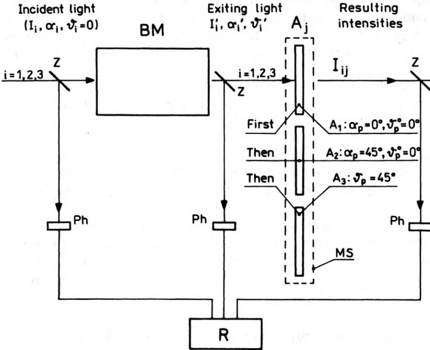
Fig. 2. Automatic system measuring the birefringent properties of the medium.  $I_i, I_i', I_{ij}$  – light intensities,  $\alpha_i, \alpha_i'$  – azimuths,  $\vartheta_i, \vartheta_i'$  – ellipticity angles, EM – examined birefringent medium,  $A_j$  – analysers, MS – measuring system for polarization state determination, Ph – photodetectors, Z – mirrors, R – recording and data processing unit
