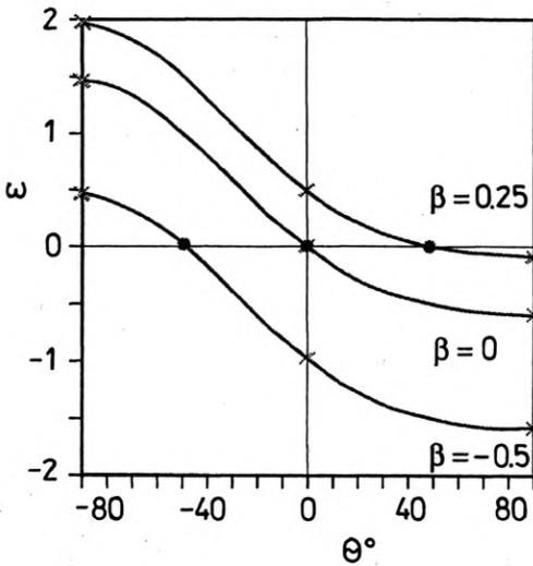
Fig. 1. Rotation frequency  $\omega$  of the polarization ellipse vs. ellipticity  $\theta$  for the centre of the pulse. The values indicated by crosses are obtained analytically. The parameter  $q_2 + \beta = 1$  is fixed
