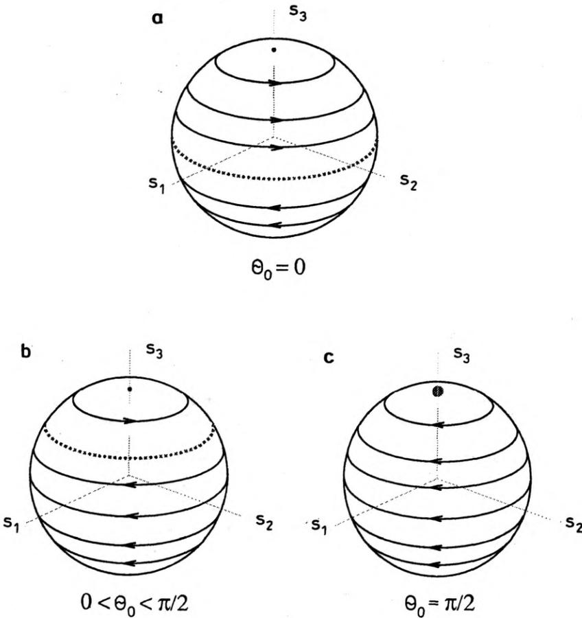
Fig. 2. Three different sets of the stationary solutions on the Poincaré sphere with (a) linear, (b) elliptic, and (c) circular polarization. The trajectories with rotating polarization ellipse are shown by solid lines. The arrows indicate the direction of the rotation
