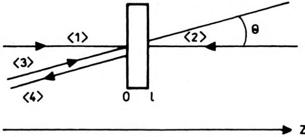
Fig. 1. Geometry of degenerate four wave mixing experiment
