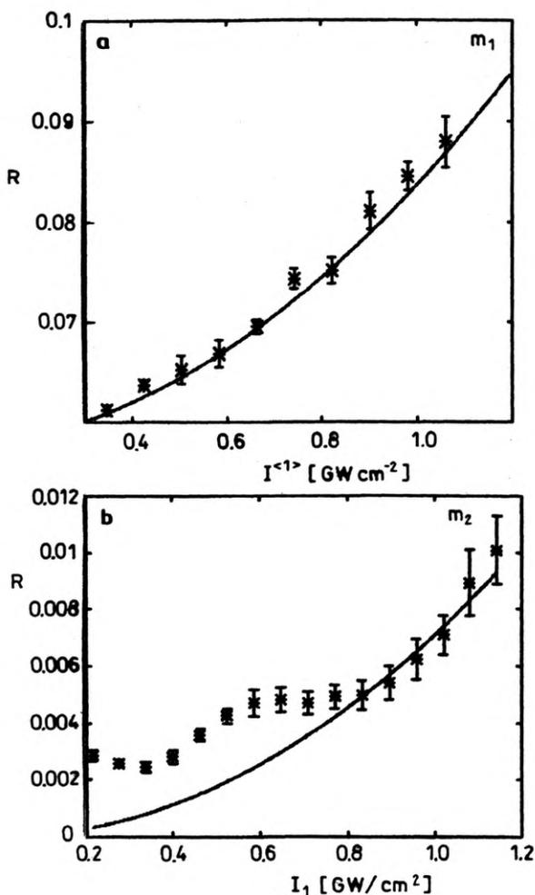
Fig. 3. Reflectivity  $R$  with respect to the pump intensity  $I^{<1>}$  reference for: **a** – the compound  $m_1$  at the optimum concentration  $C_{opt} = 9 \text{ gl}^{-1}$ , **b** – the compound  $m_2$  at the optimum concentration  $C_{opt} = 1 \text{ gl}^{-1}$ . The linear polarization states of incident beams are the same. The smooth curve represents the theoretical curve obtained from Eq. (2)
