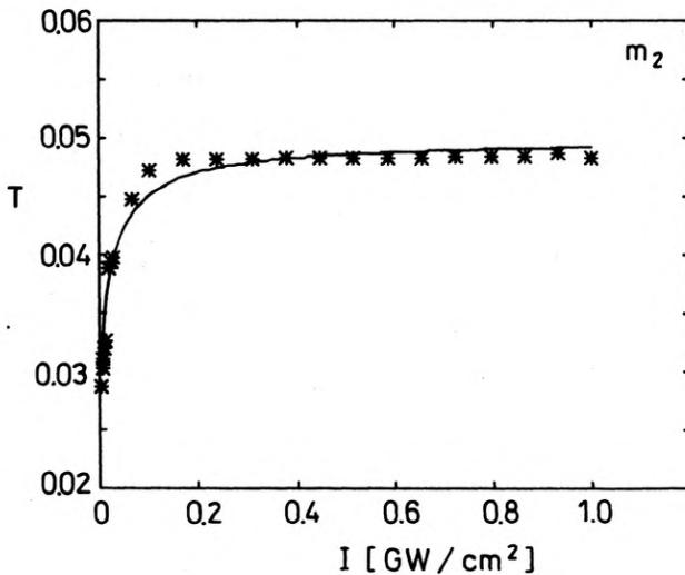
Fig. 2. Changes in the pump transmission versus pump fluence at zero delay for  $m_2$ . The sample thickness is  $l = 1$  mm. The concentration in tetrahydrofuran is 1 g/l. Asterisk represents the experimental data and the solid curve represents a fit with the solution of Eq. (1)
