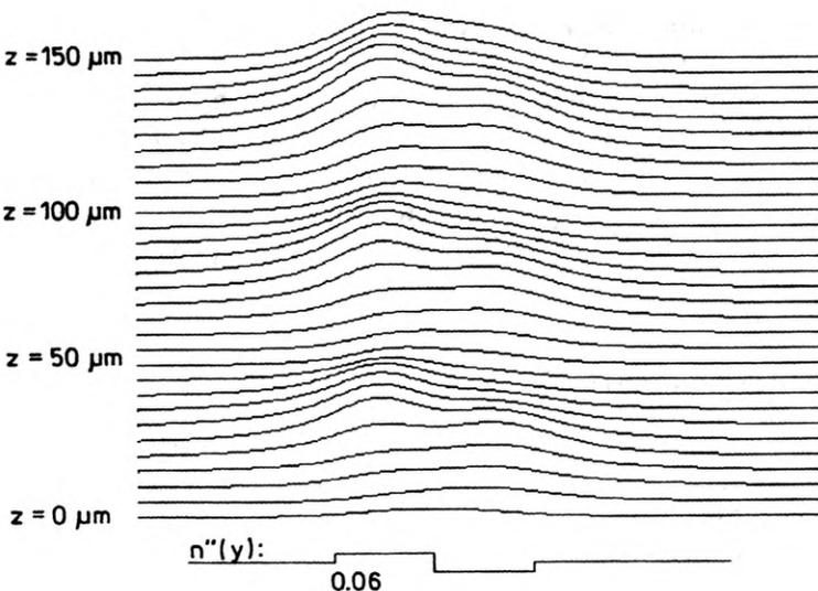
Fig. 5. Field evolution along the waveguide (BPM simulation), for  $\alpha < \alpha_{\text{branch}}$
