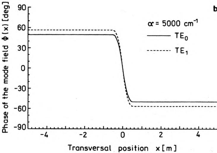
Fig. 3. Modal field and phase distributions for  $\alpha = 5000 \text{ cm}^{-1}$  (below  $\alpha_{\text{branch}}$ )
