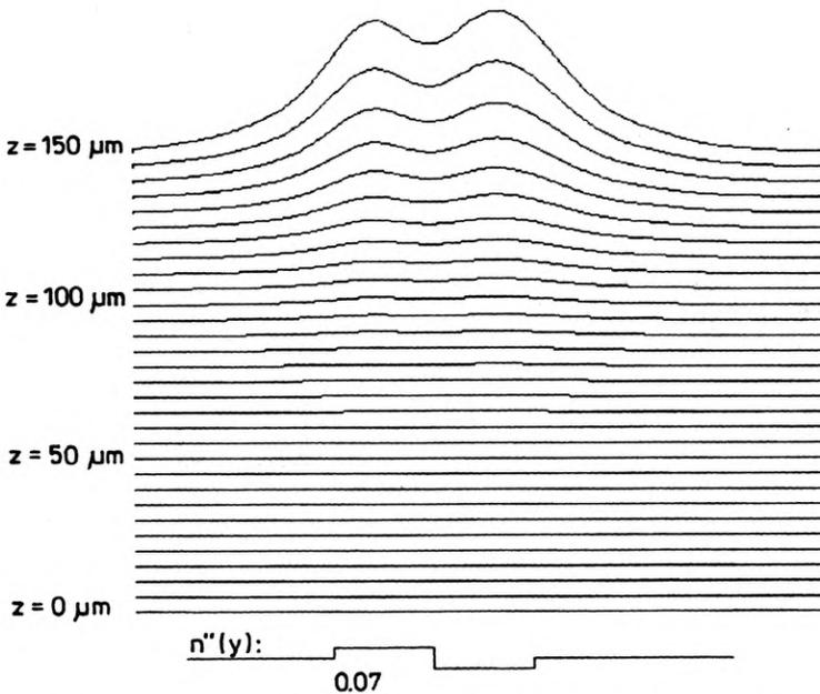
Fig. 6. Field evolution along the waveguide (BPM simulation), for  $\alpha > \alpha_{\text{branch}}$
