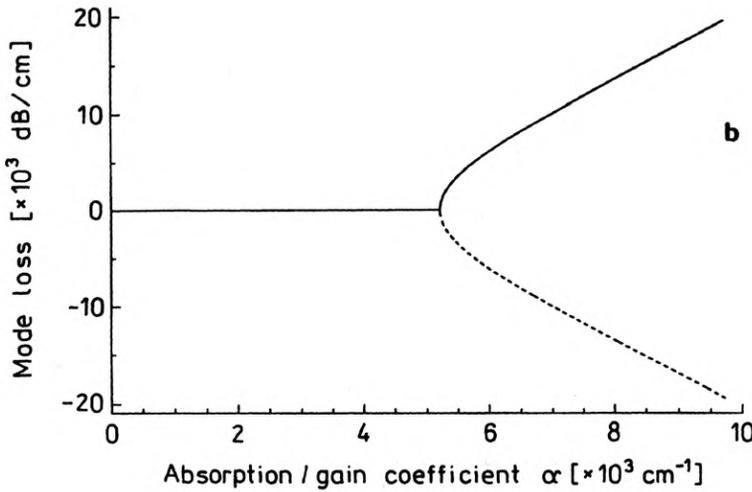
Fig. 2. Effective refractive indices  $\text{Re}\{N_{\text{eff}}\}$  and  $\alpha_{\text{eff}} = (4\pi/\lambda)\text{Im}\{N_{\text{eff}}\}$  versus  $\alpha$
