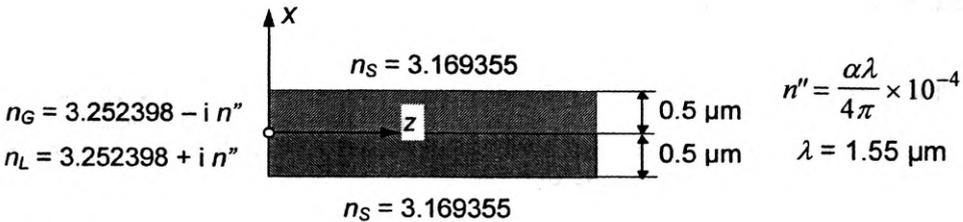
Fig. 1. Two-layer waveguide with gain and loss
