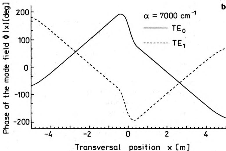
Fig. 4. Modal field and phase distributions for  $\alpha = 7000 \text{ cm}^{-1}$  (above  $\alpha_{\text{branch}}$ )
