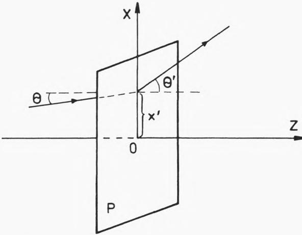
Diffraction of the ray at an optical diffracting plane  $P$ .  $\theta$  and  $\theta'$  are the incident and diffracting angles, respectively. The relationships between the direction cosines of the incident and diffracted angles are:  $l = \cos\alpha = \sin\theta$ ,  $l' = \cos\alpha' = \sin\theta'$
