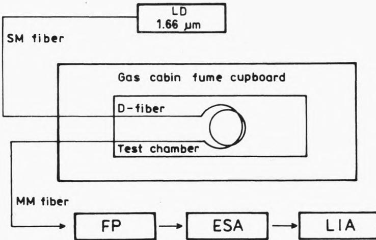
Fig. 7. Block diagram for detection of methane gas using D-fiber
