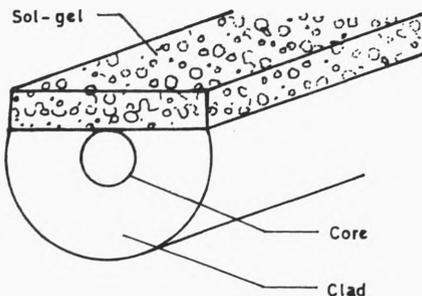
Fig. 6. Sol-gel coating for fiber optic intrinsic sensing
