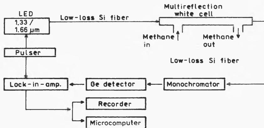
Fig. 1. Block diagram of an optical system for remote detection of CH<sub>4</sub> gas based on optical absorption method
