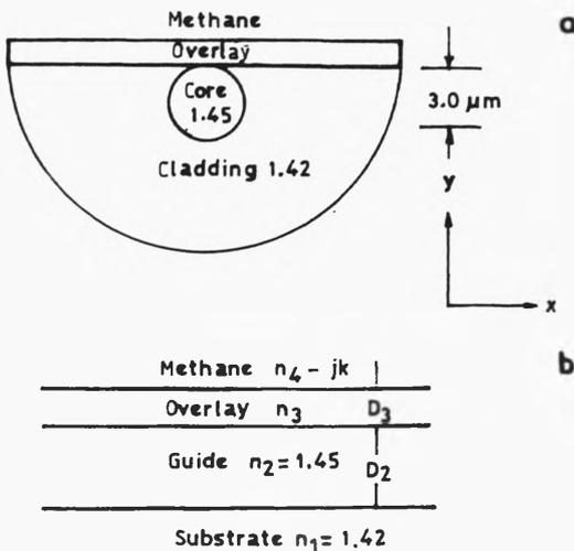
Fig. 8. Cross-section of overcoated D-fiber used for methane detection (not to the scale), (a). Overcoated planar waveguide with thin high index overlay (not to the scale), (b)
