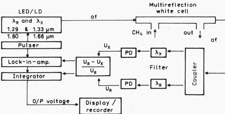
Fig. 2. Block diagram of an optical system for remote detection of  $\text{CH}_4$  gas based on differential optical absorption method
