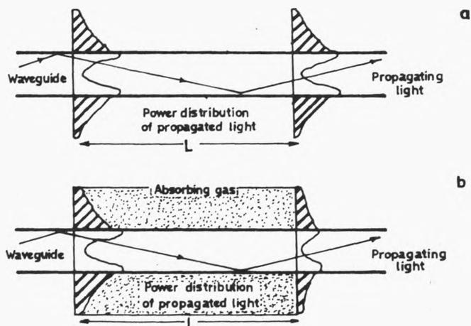
Fig. 4. Principle of detection of absorbing substance using an evanescent field. The power distribution of the propagated light through a waveguide is shown (a). When an absorbing substance, gas or liquid, surrounds the waveguide (b)
