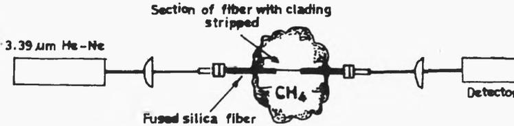
Fig. 5. Device for the detection of methane based on the attenuation of the evanescent field
