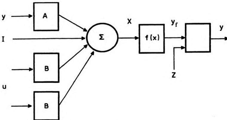
Fig. 10. Schematic of the neuron model, where:  $I$  – steering signal from neurons in the given layer,  $u$  – steering signal from neurons in other layers. If  $Z = 1$  then  $y = y_f$ , if  $Z = 0$  then  $y = 0$
