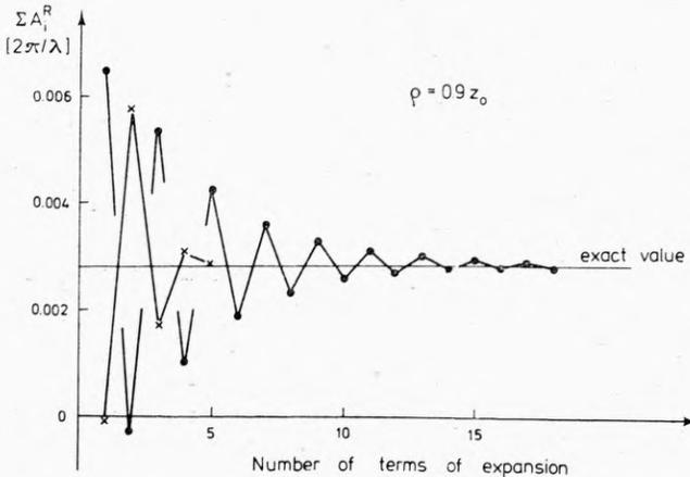
Fig. 2. Spherical aberration in the vicinity of  $\varrho = 1$  — an illustration of the increase of convergence of relations (3) and (8)
