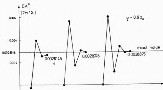
Fig. 3. Spherical aberration of the  $\Phi_R$  for  $z_c = 1.2 z_0$  and  $z_r = 1.1 z_0$  computed from the relation (8) by taking into account of the four, five and six terms of the expansion
