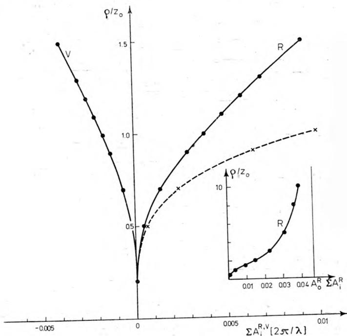
Fig. 1. Spherical aberration of wavefront  $\Phi_R$  and  $\Phi_V$  for  $z_c = 1.2 z_0$ ,  $z_r = 1.1 z_0$ ;
