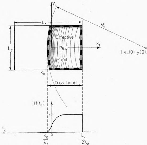
Fig. 3. Analogy between isoplanatic HOS and band-pass filter; transfer function  $H$  is shown for  $f_y = 0$
