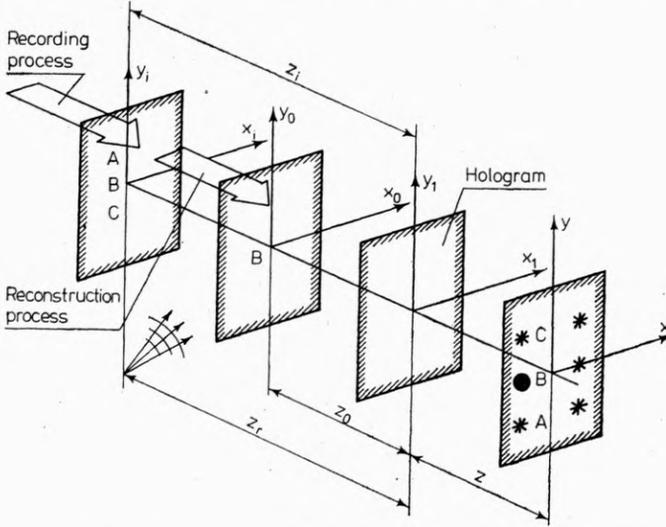
Fig. 4. Geometry of generalized Vander-Lugt filter
