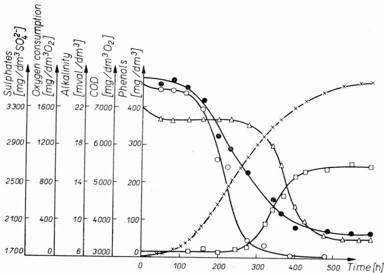
Fig. 5. Biological treatment of wastewater from wet dedusting. Dilution with municipal wastewater 9:1
