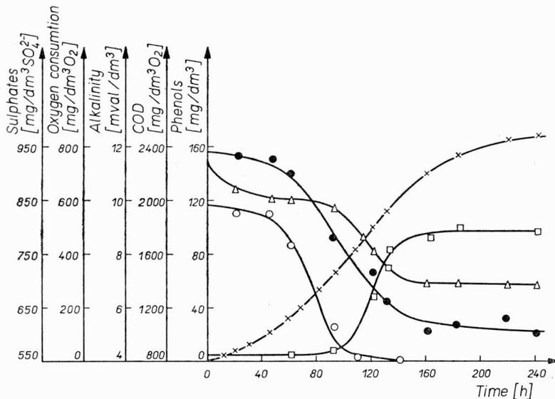
Fig. 3. Biological treatment of wastewater from wet dedusting. Dilution with municipal wastewater 1:3
