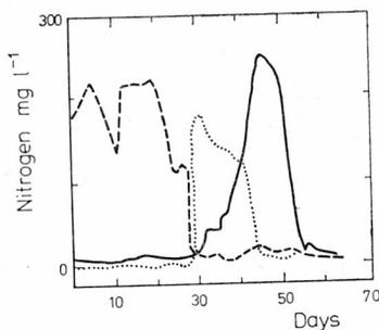
Fig. 6. The development of nitrification in aerated pig waste — — — —  $\text{NH}_4^+ - \text{N}$ , .....  $\text{NO}_2^- - \text{N}$ , ———  $\text{NO}_3^- - \text{N}$
