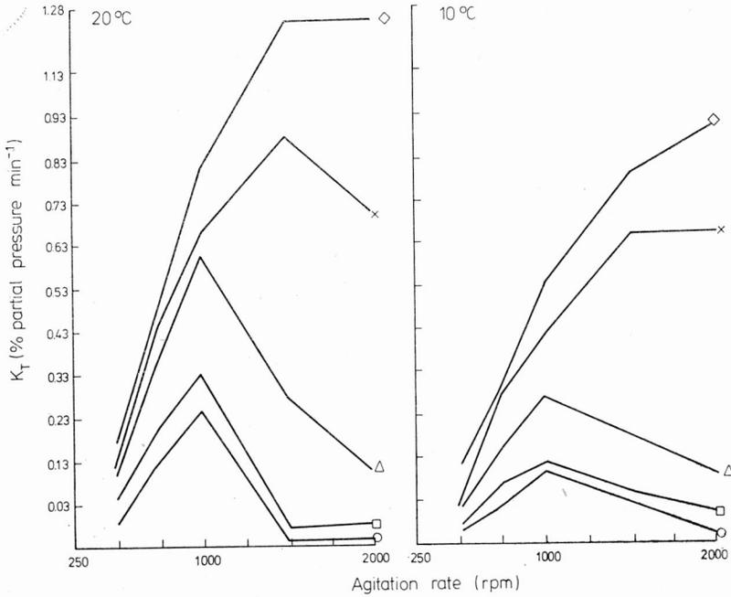
Fig. 4. Comparison of aeration, agitation, and temperature on oxygen transfer in a fermenter.
