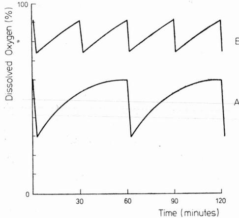
Fig. 3. Fluctuation of dissolved oxygen with loading frequency [2]
