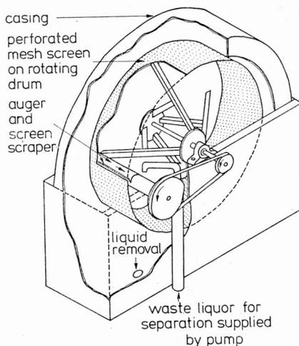
Fig. 2. Cutaway sketch of rotary screen solids separator
