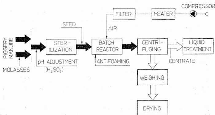
Fig. 1. Layout of batch experiment procedures
