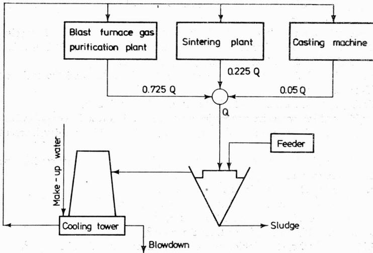
Fig. 2. The diagram of joining the cycles of blast furnace gas purification plant, sintering plant and the casting machines into integrated system
