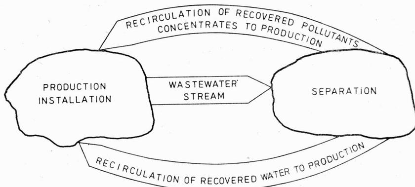
Fig. 1. Full recycling of wastewater constituents to technological process
