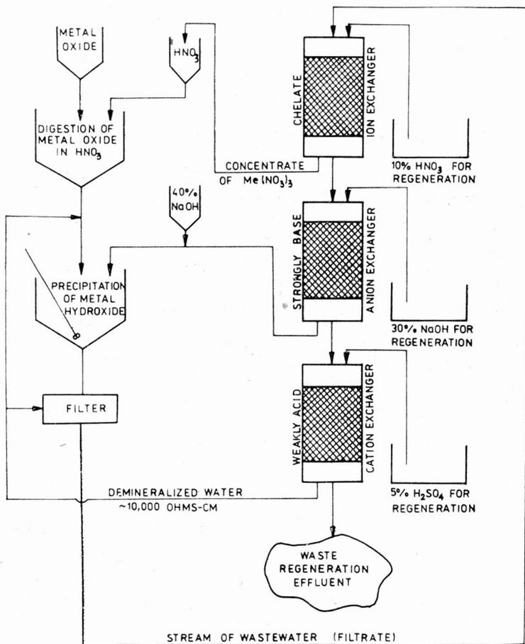
Fig. 6. Recycling of all constituents of wastewater from processing of active metal oxides to technological process by ion exchange method
