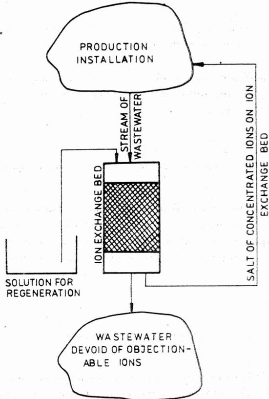
Fig. 2. Recycling of selected wastewater constituents to technological process by ion exchange method
