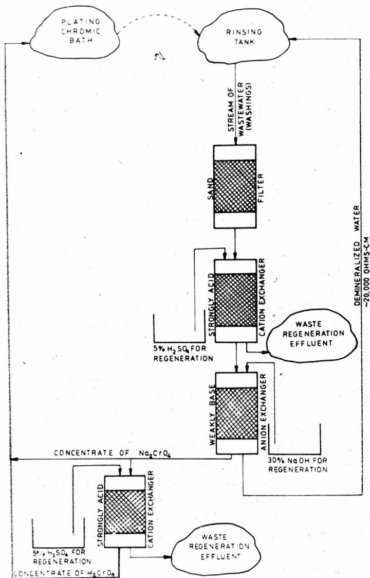
Fig. 7. Recycling of water and chromates or chromic acids from wastewater of plating plant effluent to technological process by ion exchange method
