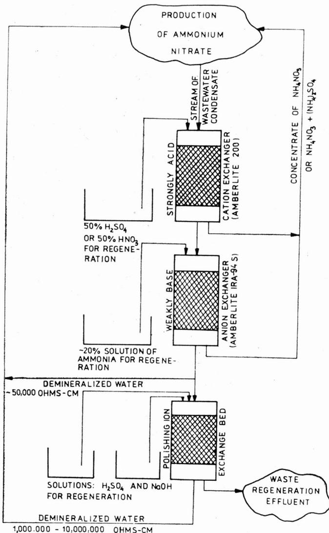
Fig. 4. Recycling of ammonia, nitrates and water from wastewater of ammonium nitrate processing to technological process by ion exchange method
