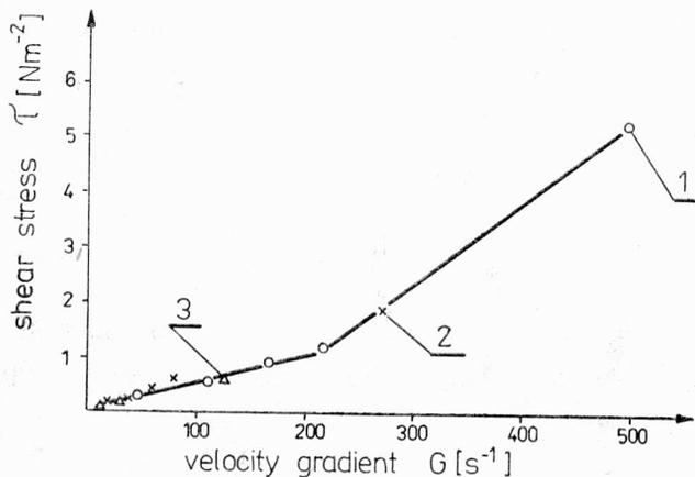
Fig. 1. The effect of velocity gradient on shearing stresses
