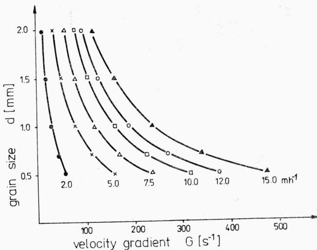
Fig. 2. Velocity gradient and filtration rate versus the grain-size of sand filter
