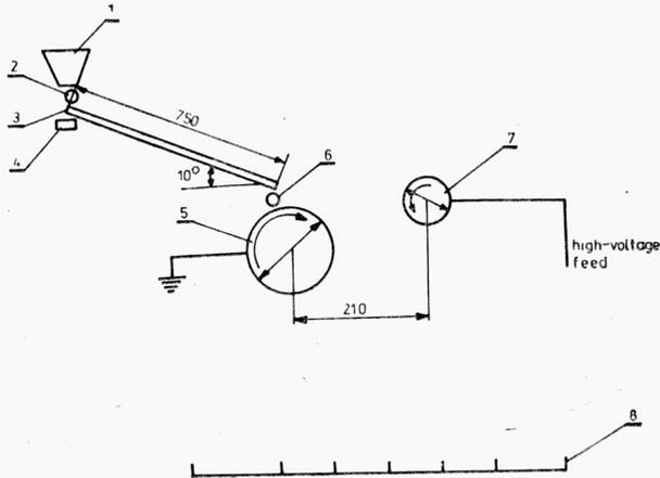
Fig. 1. Electrostatic separator
