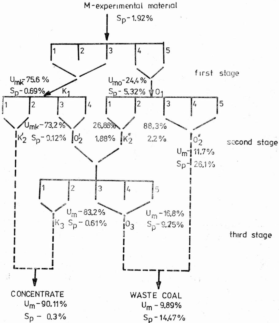
Fig. 2. Multi-stage process of bituminous coal enrichment
