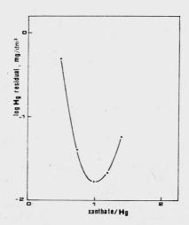
Residual mercury versus xanthate: mercury molar ratio in absence of chlorides at pH 2 and initial mercury concentration  $10~\rm mg/dm^3$
