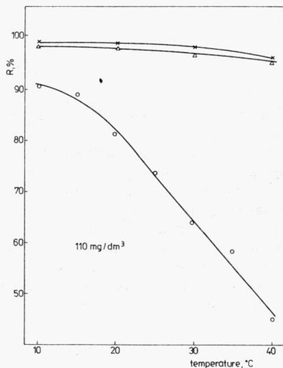
Fig. 2. Retention of dye in different temperatures.
