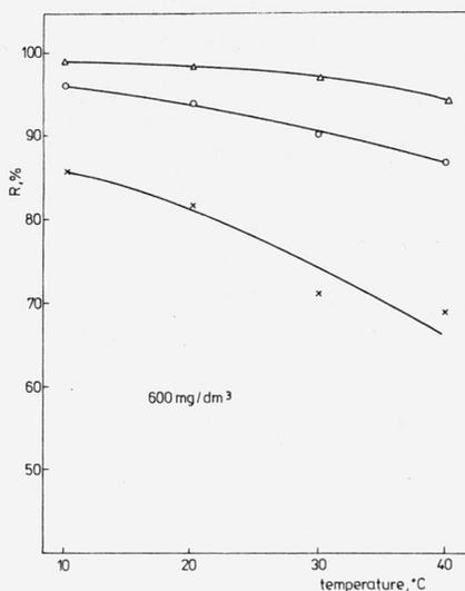
Fig. 3. Retention of dye in different temperatures. Bulk solution concentration —  $600 \text{ mg/dm}^3$
