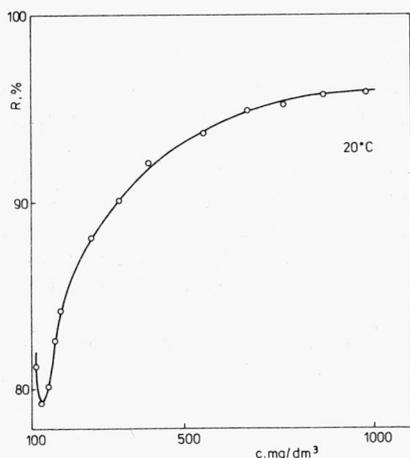
Fig. 1. Retention vs. feed solution concentration
