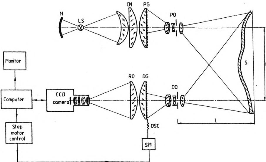
Fig. 1. Schematic representation of the projection moire system. LS — light source, M — mirror, CN — condenser, PG — projection grating, PO — projection objective, OB — object under test, DO — detection objective, DG — detection grating, RO — relay optics, SM — system motor, DSC — driving screw control
