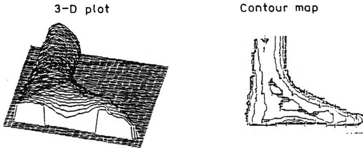
Fig. 5. 3-D plot and a contour map of the foot (lateral view) obtained by the grid projection and SCPS methods (courtesy of M. Kujawińska)
