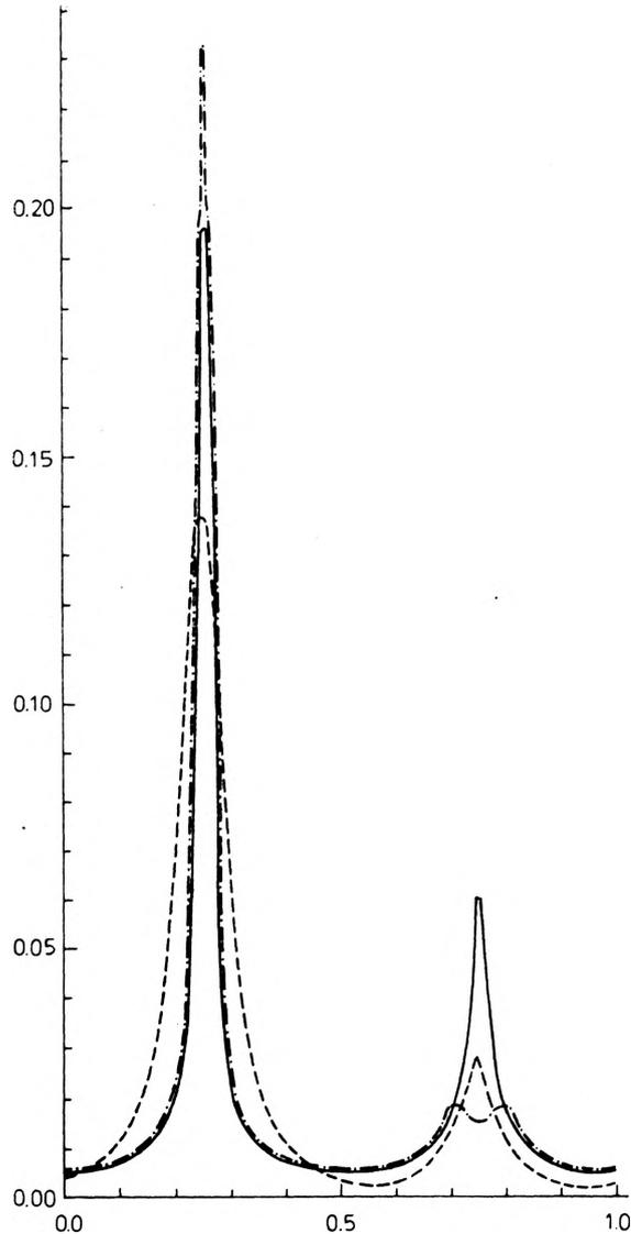
Fig. 4. Intensity curves calculated for the observation plane at the distance  $D = M + 0.5$  from the grating for three opening ratio values  $B$
