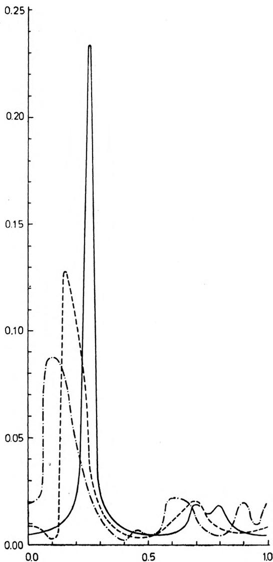
Fig. 5. SSB Fresnel diffraction intensity curves for the grating of opening ratio  $B = 0.48$ . The curves are calculated for two neighbouring planes of the characteristic plane  $D = M + 0.5$
