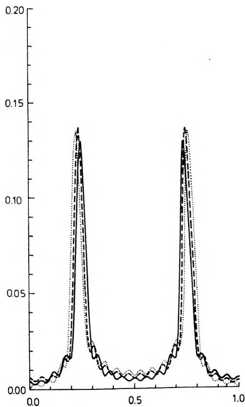
Fig. 3. Calculated intensity curves of SSB Fresnel diffraction field at the observation plane  $D = M$  for three different grating opening ratios  $B$
