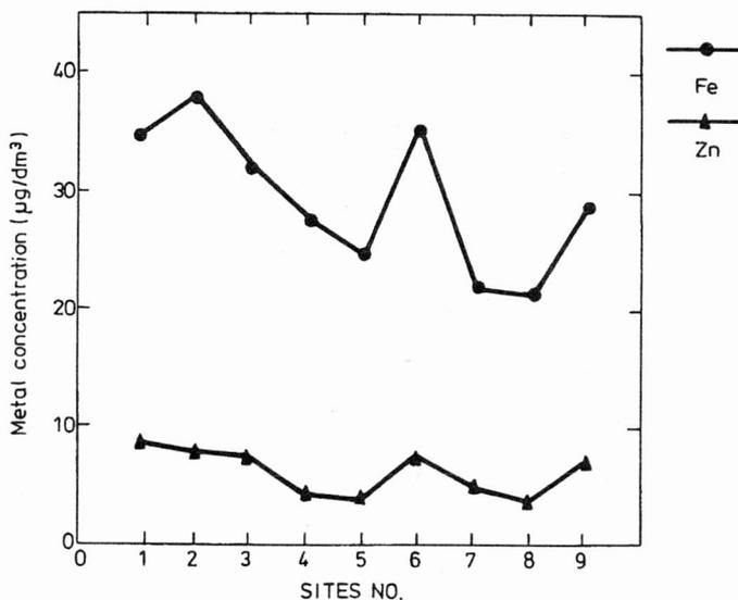
Fig. 2. Variations in mean concentrations of iron and zinc in the lake water at different sites ( $\mu\text{g}/\text{dm}^3$ )
