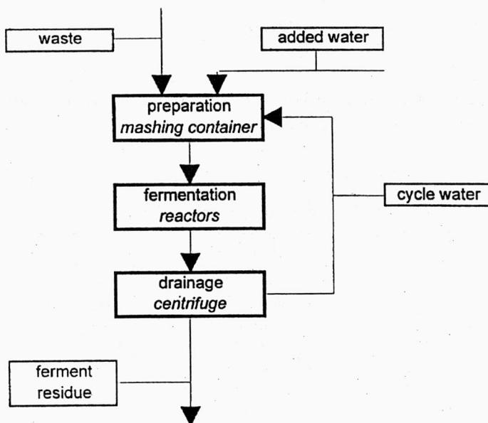
Fig. 1. Block circuit diagram of the semi-technical tests
