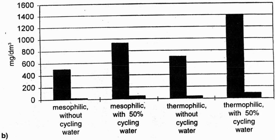
Fig. 3. Composition of process water without and with a 50% cycle of process water
