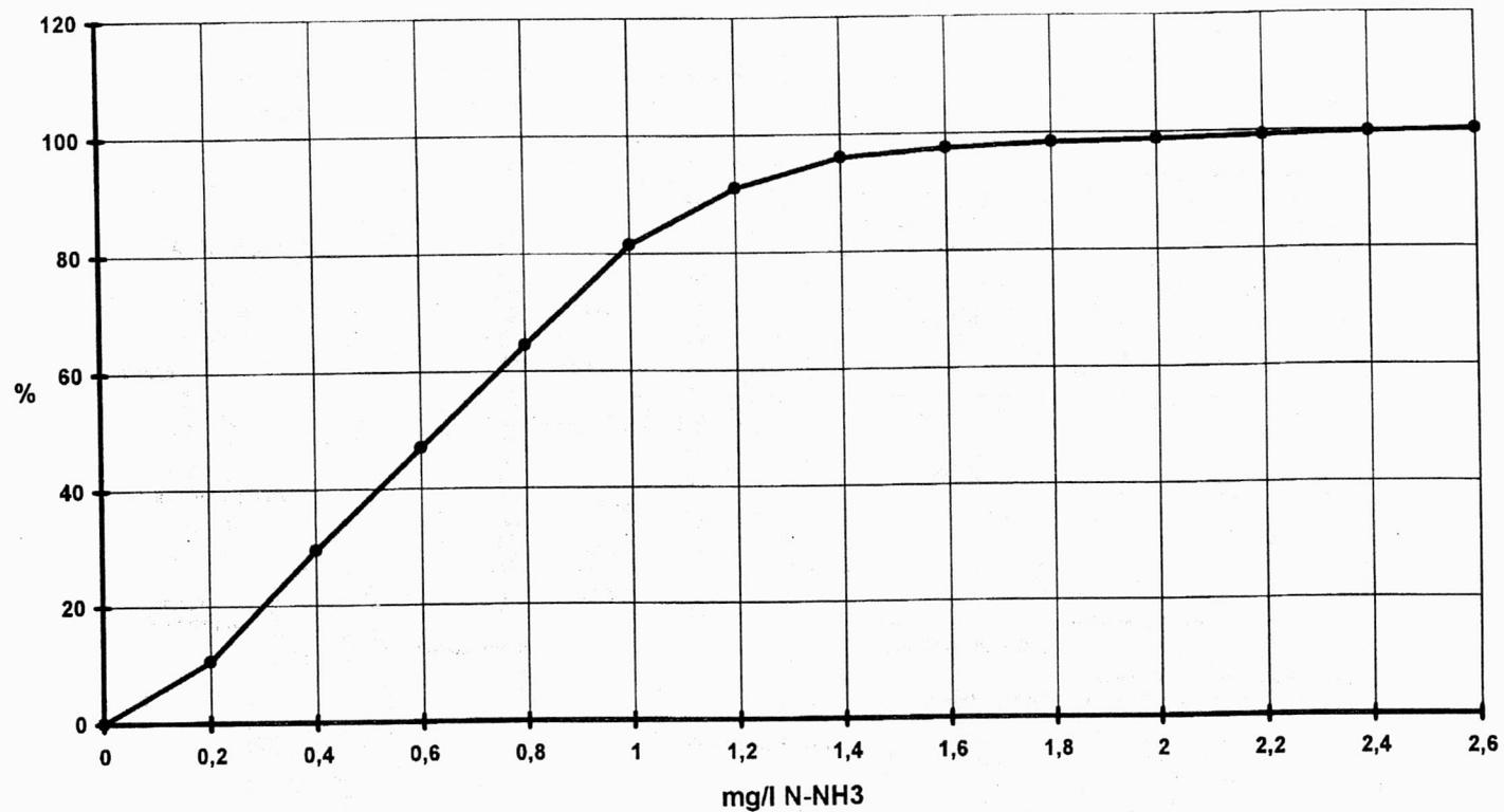
Fig. 2. Cumulative frequency of ammonium nitrogen discharged by the sewage plant Gotha in 1994 [9]
