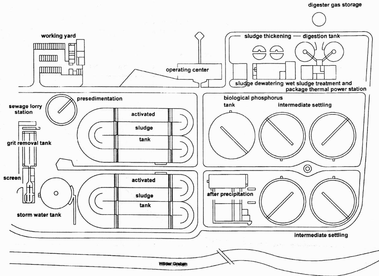
Fig. 1. Diagram of the sewage plant Gotha [9]
