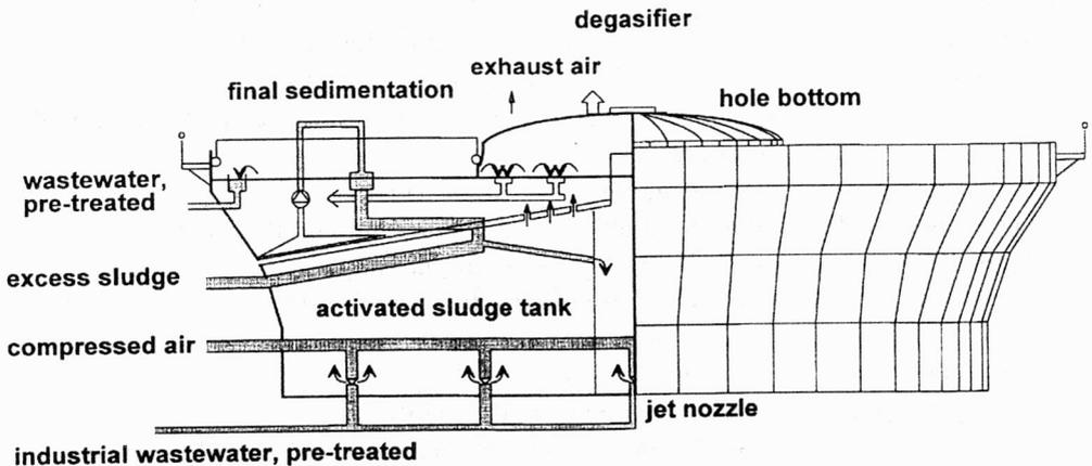
Fig. 3. Diagram of a BIOHOCH-reactor at the sewage plant Bitterfeld-Wolfen [7]
