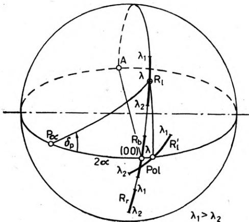
Fig. 5. Illustration of the transformation of the polarization states of the light waves creating the spectrum  $R_l$  of the left hand image of the stria for the azimuth of the phase plate  $P$  different from zero
