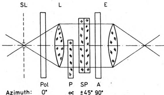
Fig. 1. The observing telescope of the striascope with the Savart polariscope and the azimuthal compensating plate: *SL* - plane of the exit slit of the striascope, *Pol* - polarizer, *P* - phase plate acting as the azimuthal compensator, *SP* - Savart plate, *A* - analyzer, *L* - lens creating the image of the striae in the object plane of the ocular, *E* - eyepiece
