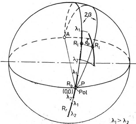
Fig. 4. Illustration of the transformation of the polarization states of the light waves creating the spectrum  $R_l$  of the left hand image of the stria under the zeroth azimuth ( $\alpha = 0$ ) of the phase plate. The angular distance  $2\beta$  of the representation of the polarization state for an arbitrary wavelength  $\lambda$  before and after the transformation from the point  $A$  representing the azimuth of the analyzer remaining constant
