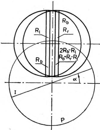
Fig. 3. Rotation of the phase plate by an angle  $\alpha$  causes the transfer of the background colour on one image of the striae. The background colour in the region uncovered by the compensating phase plate  $P$  plays the part of the reference colour.  $I$  - direction of the oscillation of the electric field strength vector of the faster wave in the plate
