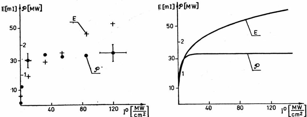
Fig. 5. Energy and power of the pulse emerging from the two-component system as a function of intensity of the input pulse.
