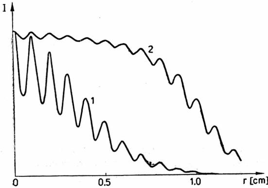
Fig. 8. The smoothing of the nonuniformities in the spatial distribution of radiation due to two-photon absorption.
