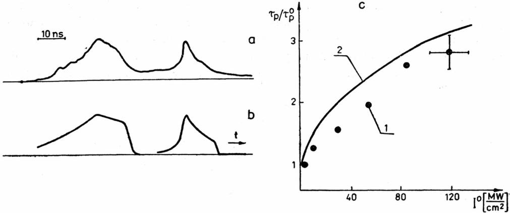
Fig. 4. Deformation of time shape of pulse in the system with two-photon absorbent obtained from experiment (a), and from calculations (b). The input pulse situated on the right hand side. c – dependence of the pulse length at the output upon the input pulse intensity:
