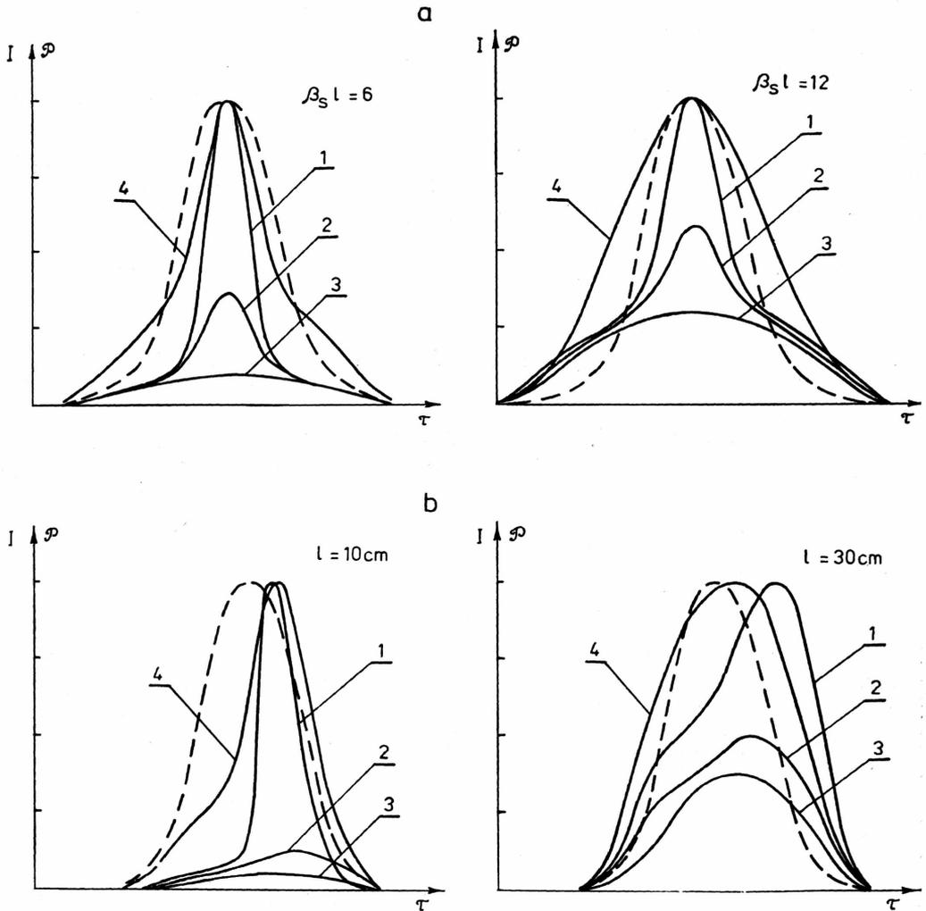
Fig. 2. Time deformation of the both power (4) and intensity (1, 2, 3) distributions of radiation at different distances from the Gaussian beam axis for the case of quasi-stationary (a), and nonstationary (b) interaction with two-photon absorbent. 1 -  $r = 0$ , 2 -  $r = 3/5 r_0$ , 3 -  $r = 6/5 r_0$ . Broken line denotes input distribution
