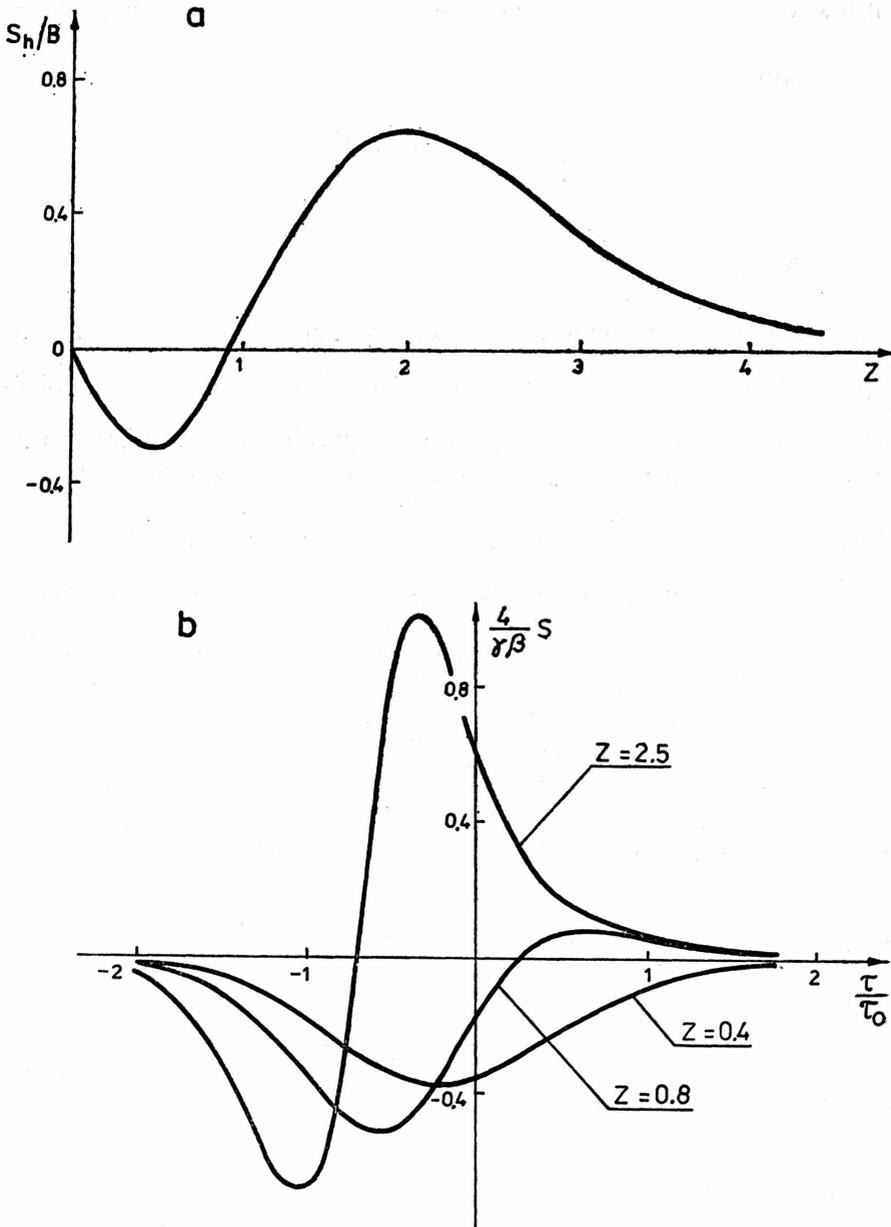
Fig. 7. The function of spatial compression in two-photon absorbent in the case of nonstationary interaction. a — relative speed of changes in the intensity distribution width as a function of intensity on the axis. b — relative speed of change in the intensity distribution at various time moments  $\tau$
