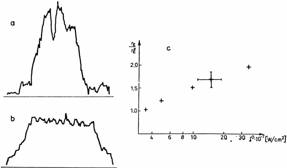
Fig. 9. The densitograms of the spatial distribution of the radiation energy density at the input (a), and output (b) of the GaAs plate and the dependence of the effective width of the output distribution upon the intensity (c) of the picosecond pulse
