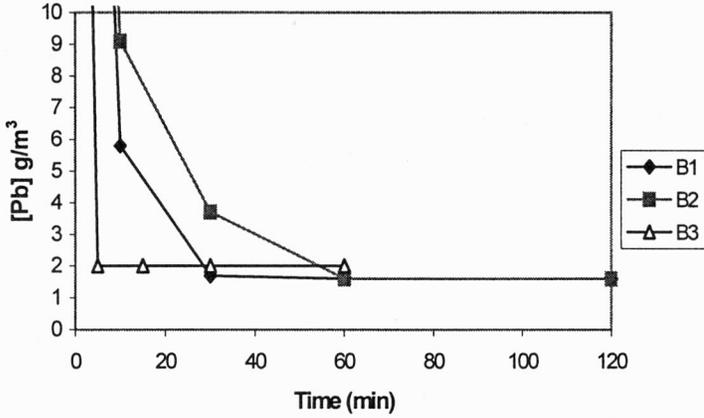
Fig. 1. [Pb] vs. time for three types of iron ( $[Pb] = 40 \text{ g/m}^3$ ) [3], [5]
