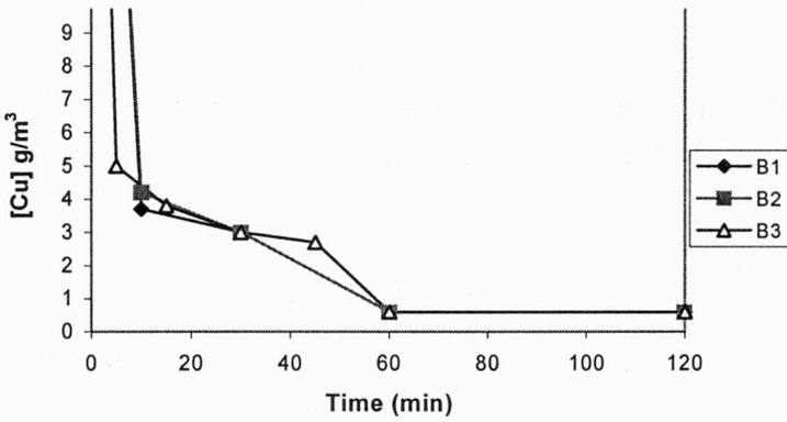
Fig. 2. [Cu] vs. time for three sources of iron ( $[Cu] = 30 \text{ g/m}^3$ ) [3], [5]
